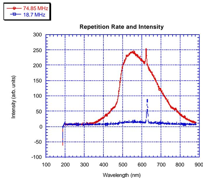
Figure 9: Effects of repetition rate on intensity.
