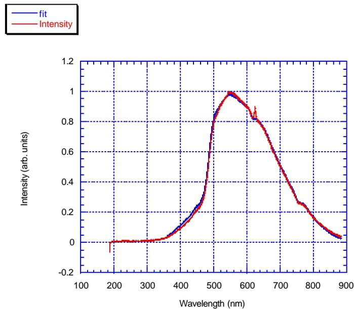
Figure 6: Carbon target ablated by FEL at 500 W (red), and corrected blackbody curve for  $T=3100$  K (blue). Intensity has been normalized to 1.
