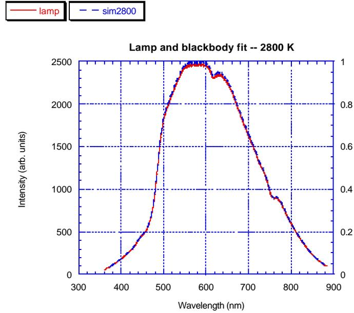
Figure 4: Spectrum (red solid) and fit to Eq. (6) (blue dashed) for a 2800-K lamp.
