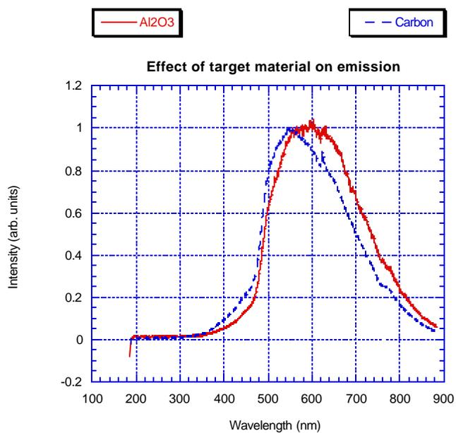
Figure 11: Effect of target material on plasma emission. Intensity has been normalized to same maximum value
