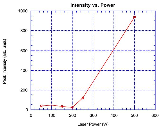
Figure 7: Peak intensity versus laser power for carbon target ablation.
