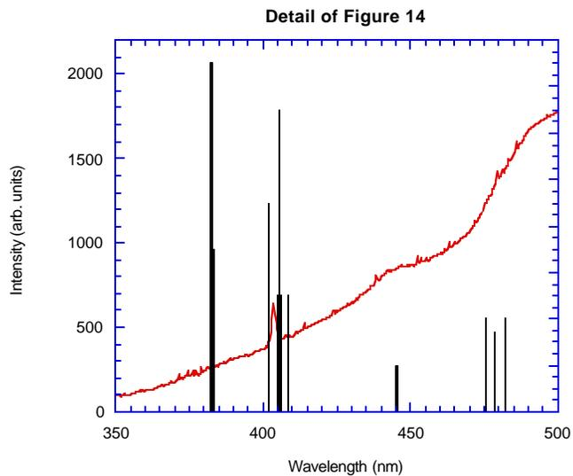
Figure 15: Detail of Figure 14 showing emission spike at ~405 nm for FeMn emission curve (red).
