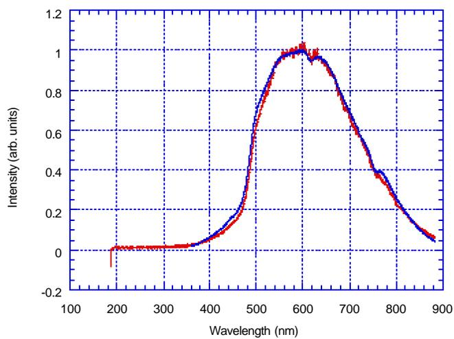
Figure 12: Emission spectrum (red) and fit from Eq. (6) (blue) for Al<sub>2</sub>O<sub>3</sub> target in Figure 11.
