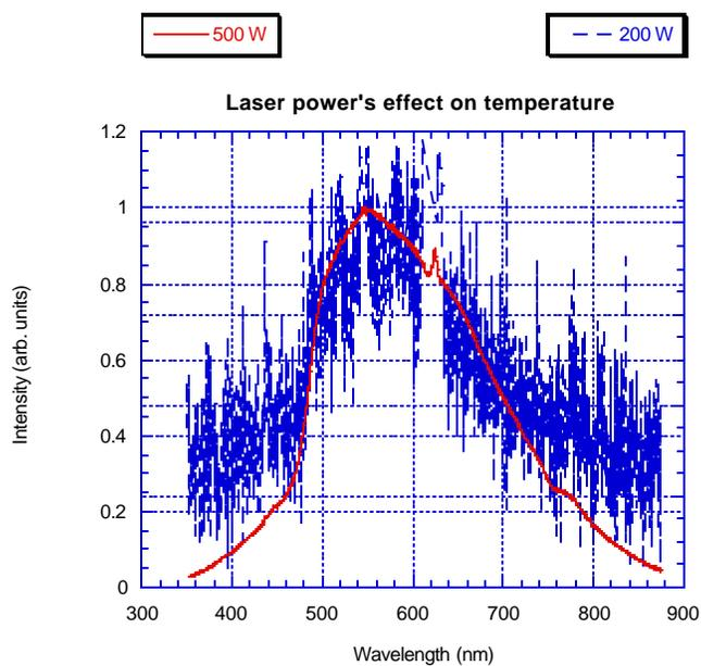
Figure 8: Effect of laser power on temperature. Approximate blackbody curves shown. Sharp peaks in 200 W curve are reflections of the FEL harmonics. Both curves have been normalized in intensity to the same maximum value.
