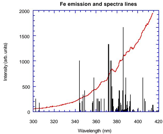
Figure 13: Emission spectrum from Fe target (red) with spectral lines due to emission from Fe neutrals and singly ionized states overlaid (black).
