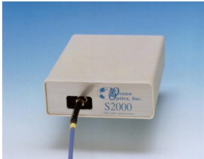
Figure 2: Ocean Optics S2000 spectrometer, exterior
