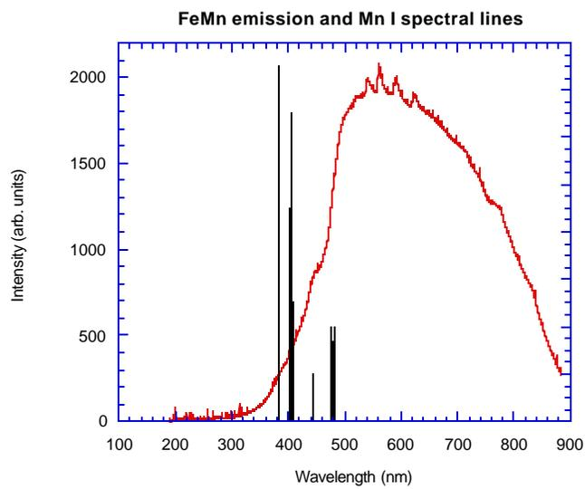
Figure 14: Emission spectrum from an FeMn target (red) with Mn neutral emission spectral lines overlaid (black).
