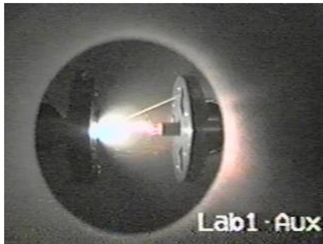
Figure 3: Laser ablation taking place inside vacuum chamber. Notice the white plume from the target on the left.
