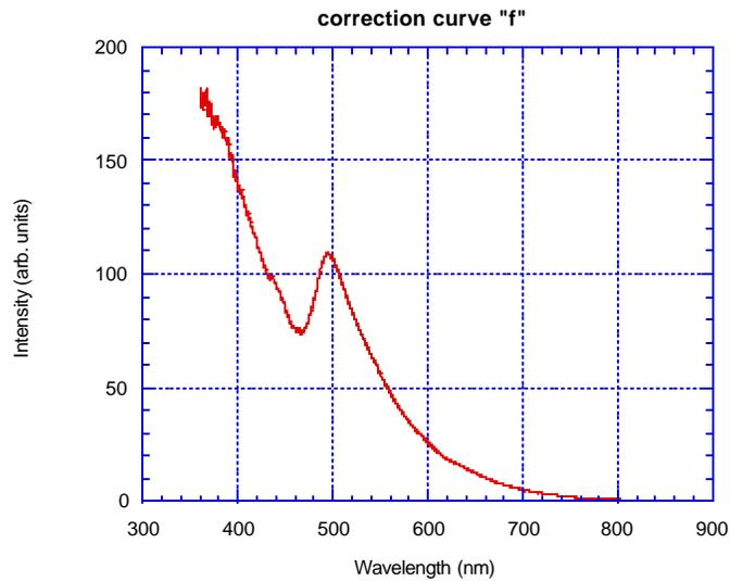
Figure 5: Correction function  $f$  from Eq. (6) taken from fit of 2800 K lamp spectrum.
