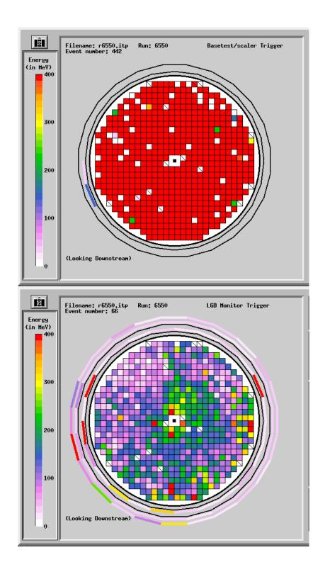
Figure 7: The LGD depiction of base test and LGD monitor events with lines through blocks labeled dead by the algorithm.
