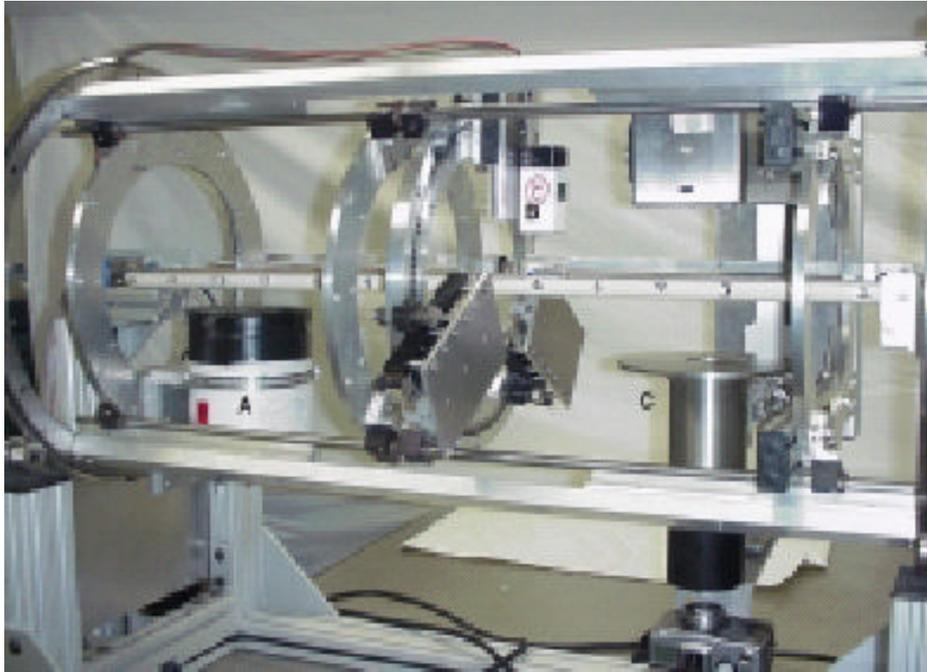
**Figure 5:** Picture of the new gantry being developed for SPECT imaging
