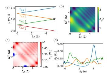
FIG. 2. (a) Drift velocities versus  $\Delta_Z$  for  $\theta_v=0$ ,  $\Delta_v=\tilde{\epsilon}_F/2$ , and  $\tilde{\epsilon}_F=10~\Delta$ . (b)  $T_{he}$  versus  $\Delta_Z$  and  $\Delta_v$  for  $L_{sc}=0.9~\xi,~v_{s,s}=0.1\Delta\xi/\hbar$ , and  $k_F=5\hbar/\xi$ . (c)  $R_D$  corresponding to panel (b). (d) Line cuts of  $R_D$  for fixed  $\Delta_v=(0,~2.5,~5)\Delta$ , blue, orange, green, traces, respectively. Stars denote the values of  $R_D$  when  $\Delta_Z=\Delta_v$ .
