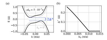
FIG. 4. (a) Spectrum for effective 1D model with finite superconducting pairing  $\Delta$  and small offset  $k_0$ . (b) Topological gap  $\Delta^*$  as a function of  $k_0$  for a fit corresponding to  $\theta = \pi/4$ .
