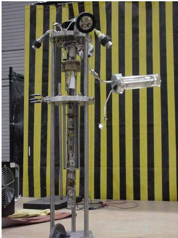
Figure 2.22: The target stick connected to a vacuum flange (with feedthroughs) for vertical insertion into the EG1 target system.
