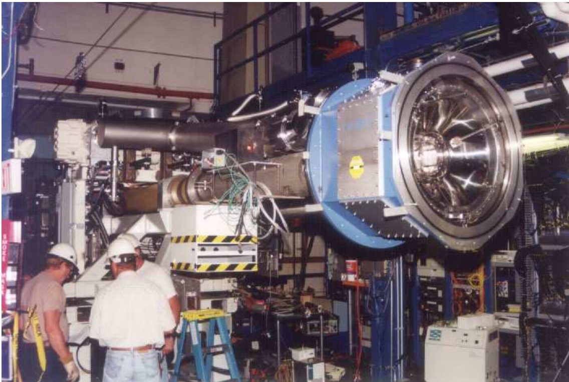
Figure 2.26: The assembled EG1 polarized target, viewed downstream, prior to insertion into CLAS.
