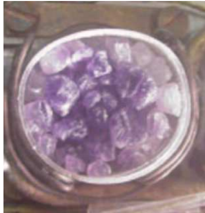
Figure 2.13: Beads of ammonia in a target cup. The purple discoloration is due to radiation damage.
