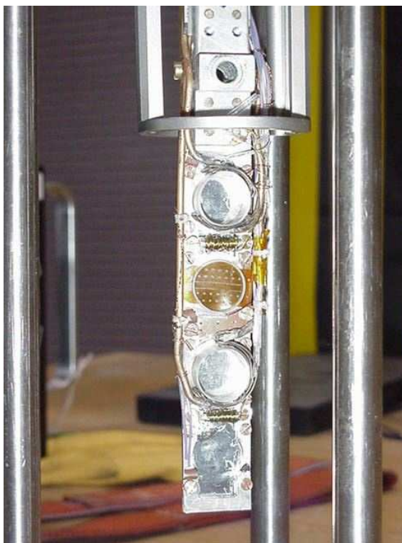
Figure 2.21: Target insert strip showing the 4 target cells used for the EG1 targets: \text{ND}_3 , ^{12}\text{C} , \text{NH}_3 and empty, from the top down. Note the NMR coils that surround the \text{ND}_3 and \text{NH}_3 cells. Only the carbon target is full at the time of this photograph.
