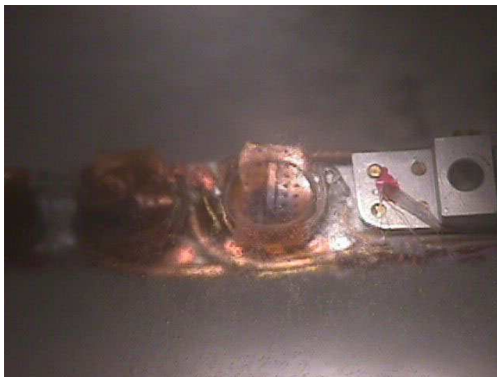
Figure 2.23: The target stick, all cells filled, immersed in a liquid nitrogen bath. The \text{NH}_3 cell is shown.
