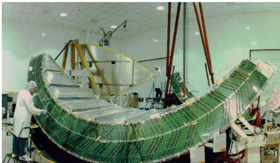
Figure 2.31: Photograph of one sector of an outer layer drift chamber section prior to installation in the CLAS detector. From the JLab JPIX picture exchange.
