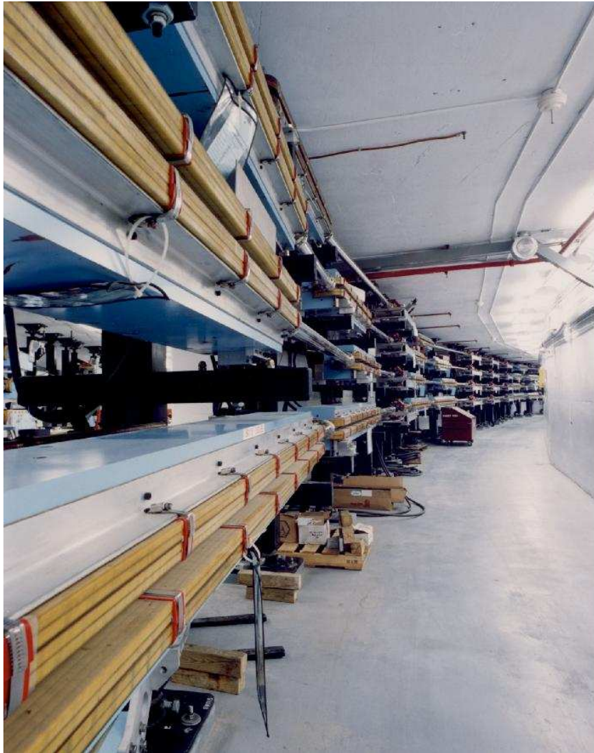
Figure 2.6: Photograph of a section of a recirculation arc. From the JPIX Jefferson Lab picture exchange.
