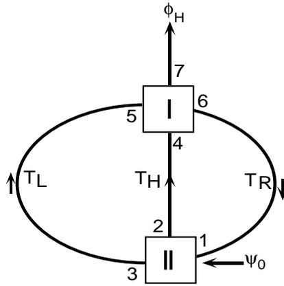
**FIGURE 2.** Diagram of the possible paths a disturbance may take as it propagates from the antenna input,  $\psi_0$ , to the output hybrid channel,  $\phi_H$ . The resulting steady state field set up by the antenna is a linear superposition of all possible paths through this flow diagram.
